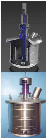
Rotating vibro-granulator is applied in the chemical industry and is intended for dispersion fusion of nitrogen fertilizers on uniform drops in the granulation tower with their following cooling and crystallization into solid granules/prills in the process of a free fall in the up-coming stream of cooling air.
