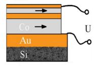
Schematic imege of the functional element of the magnetic field sensor based on the spin-valve
